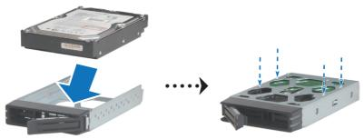
• For 2.5" Hard Disk: Place the hard disk in the hard drive tray, turn the tray upside down, and then tighten the screws to secure the hard disk.
