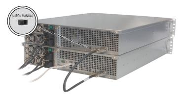
• If the AUTO/MANUAL switch is set to MANUAL, press the POWER button to turn on RX1211/RX1211RP.
