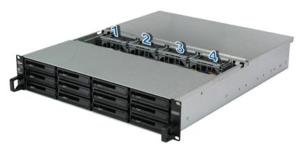
**4** Find the malfunctioning fan and lift it upward to remove.
