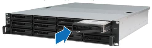
Important: Make sure the drive tray is completely inserted. Otherwise, the drive might not function properly.
