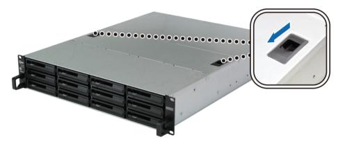
2 Lift and remove the fan cover.
