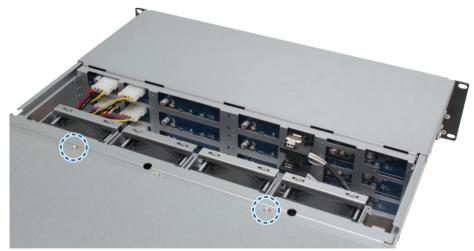
**b** Remove the two screws located on the back. Then slide the top cover in the direction indicated below and lift.
