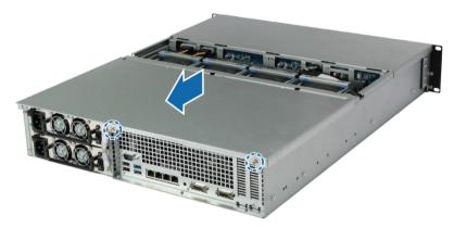
c Remove the screws of the securing bracket and remove the securing bracket to reveal the RAM slots.
