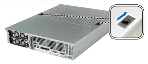
3 Lift and remove the fan cover.
