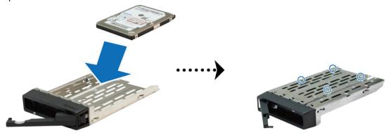
3 Insert the loaded drive tray into the empty hard drive bay.
