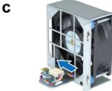
7 Slide the new cooling fan unit into the RackStation. Make sure the power port is aligned properly.
