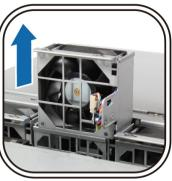
**5** Apply firm pressure to the power plug and slide it off the power port as shown below. Then remove the malfunctioning fan from the fan casing.
