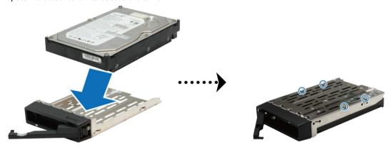
• For 2.5" drives: Place the drive in the drive tray. Turn the tray upside down and tighten screws into the four spots indicated below to secure the drive.
