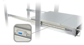
**Warning:** Before pulling the unit out of the rack, please make sure you have disconnected all the cables from your RackStation (or expansion unit). You might also need other people's help to hold the unit steady and prevent it from accidental dropping
