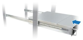
**b** When you hear a clicking sound indicating the sliding rails are locked, push the purple latches backward to unlock the sliding rails.
