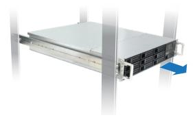
2 Push the white latch forward to unlock the sliding rails, and carefully pull the unit out of the rack.
