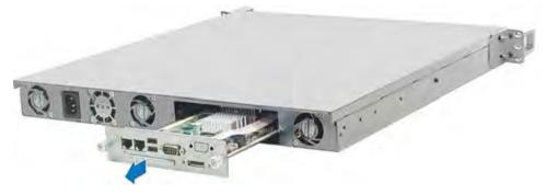
*Important:* When you pull out the panel, you expose sensitive internal components. Avoid touching anything other than the memory assembly when you remove or add memory.
