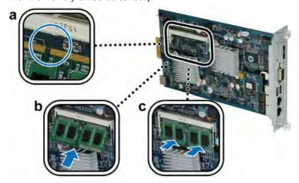
Important: Hold the memory module by its edges, and do not touch the gold connectors.
