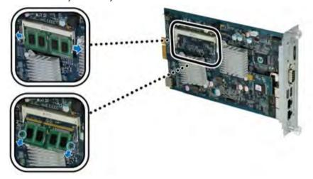
4 Follow step 5 and 6 of the "Install the RAM Module" section to replace the circuit board.
