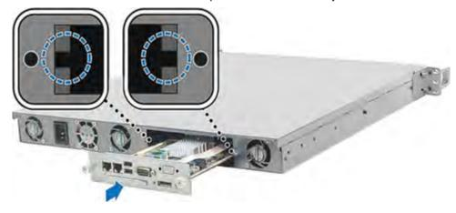
c Tighten the 2 knobs you unscrewed in step 2.
