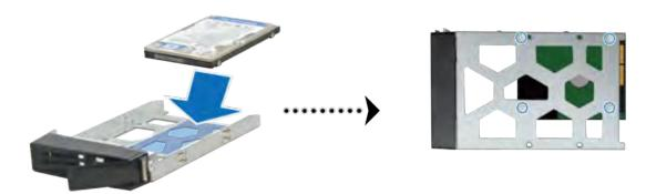
3 Insert the loaded hard drive tray into the empty hard drive bay.
