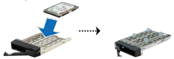
3 After securing the hard disk and tray, insert both into the empty hard drive bay.
