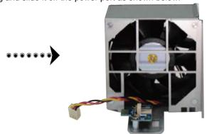
4 Remove the malfunctioning fan from the fan casing.
