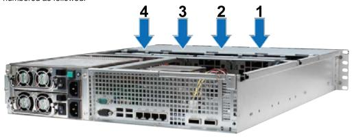
2 Find the malfunctioning fan. Lift the fan upward to remove.
