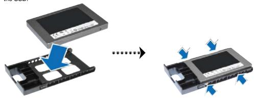
3 After securing the SSD and tray, insert both into the empty SSD bay.
