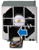
7 Slide the new cooling fan unit into your RackStation. Make sure the power port is aligned properly.
