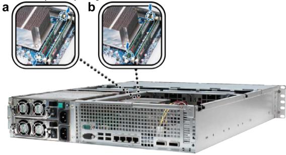
3 Replace the top cover, slide it into place, and tighten the two back screws.
