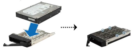
• 2.5" Hard Disk: Place the hard disk in the hard drive tray. Turn the tray upside down and tighten screws into the four spots indicated below to secure the hard disk.
