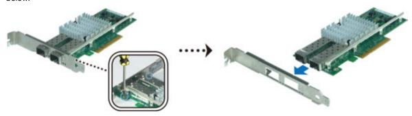
2 Replace the longer bracket with the shorter one from your RackStation. Then tighten the two screws to secure the shorter bracket.
