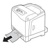
2 Remove the standard 250-sheet tray from the printer, and then pull out the jammed paper remaining inside the printer. If you cannot remove the jammed paper or cannot find any jammed paper there, go to the next step to remove the jammed paper from the inside of the printer.
