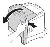
Open the belt unit until it stops and remove the jammed paper. Confirm that there are no scraps of paper remaining inside the printer.
