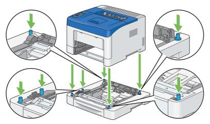
10 Secure the optional 250 sheet feeder to the printer by tightening the two screws provided with the feeder with a coin or similar object.
