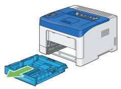
9 Lift the printer and align the five guide pins of the optional 250 sheet feeder with the holes at the bottom of the printer. Gently lower the printer onto the optional 250 sheet feeder.
