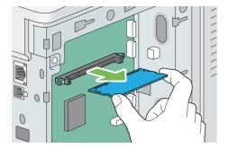
6 Align the guide on the control board cover with the slot around the control board, and slide it towards the front of the printer.
