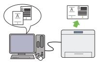
The Pages Per Sheet (N-Up) feature allows you to print multiple pages on a single sheet of paper. This feature helps reduce the paper consumption.
