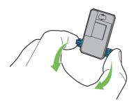
5 Hold the edge of the font ROM and the connector toward the control board, and then insert it into the slot.
