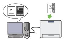
The 2-Sided Print feature is to print two or more pages on the front and back side of a single sheet of paper. This feature helps reduce the paper consumption.
