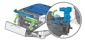
4 Make sure that the arrow marks on the transfer unit and the printer face each other, and then press the two tabs on transfer unit inward to lock.
