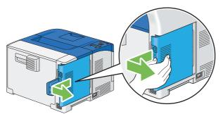
5 Remove the wireless printer adapter from the printer by releasing the adapter's hook while pushing the wireless printer adapter towards the front of the printer.
