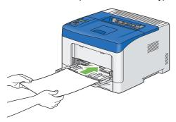
Slide both width guides until they rest lightly against the edge of the print media stack.
