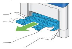
7 Pull the standard 250 sheet tray out of the printer about 200 mm.
