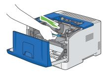
5 Grasp the handle on the top of the drum cartridge with the other hand, and then pull it out completely.
