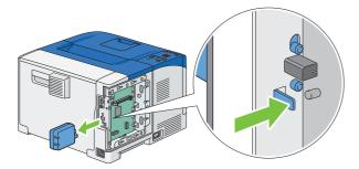
6 Align the guide on the control board cover with the slot around the control board, and slide it towards the front of the printer.
