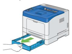
2 Hold the optional 250 sheet feeder with both hands, and remove it from the printer.
