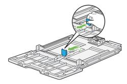
5 Load the print media into the bypass tray with the recommended print side facing up so that the top edge of the print media enters the printer first.
