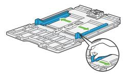
4 Pull up the length guide and slide it toward the bypass tray cover until it stops.
