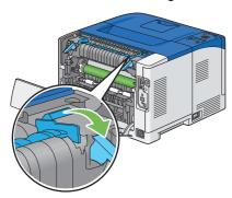
b Remove the jammed document from above the fusing unit.
