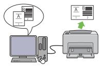
Multiple-Up enables you to print multiple pages on a single sheet of paper. This feature allows you to reduce the paper consumption.
