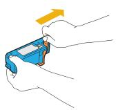
3 Adjust the toner cartridge to the associated cartridge holder, and then insert it firmly by pressing near the center of the label until the toner cartridge clicks.
