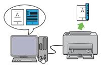
2 Sided Print is to print two or more pages on the front and back sides of a single sheet of paper manually. This feature allows you to reduce the paper consumption.
