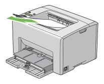
4 Remove any paper in the priority sheet inserter (PSI) or multipurpose feeder (MPF). Keep the paper wrapped and away from humidity and dirt.
