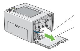
7 Insert the print head cleaning rod fully into the hole beside the arrow on the printer until its tip reaches the interior of the printer as illustrated below, and then pull it out.
