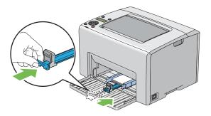
**10** Insert the PSI into the printer and then align the PSI to the marking on the MPF.
