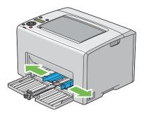
6 Before loading the print media, flex the sheets back and forth, and then fan them. Straighten the edges of the stack on a level surface.
