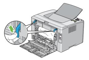
3 Remove any paper jammed from the back of the printer.
