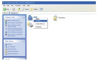
Wait for the driver information to be copied from the server computer to the client computer, and for a new printer object to be added to the **Printers and Faxes** folder. The time taken to copy varies based on the network traffic.
