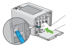
**10** Replace the black toner cartridge by adjusting it to the associated cartridge holder, and then insert it firmly by pressing near the center of the label until the toner cartridge clicks.
