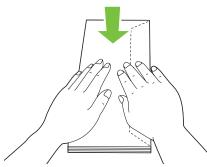
• If envelopes are still not fed correctly, add some bending to the flap of the envelopes as shown in the following illustration.
