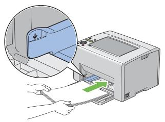
8 Adjust the paper width guides until they rest lightly against the edges of the stack of print media.
