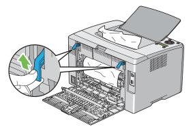
3 Remove any paper jammed from the back of the printer. If no paper is found in the paper path, then remove any paper jammed out of the center output tray.
