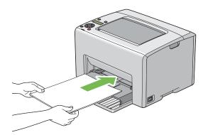
6 Adjust the paper width guides until they rest lightly against the edges of the stack of print media.
