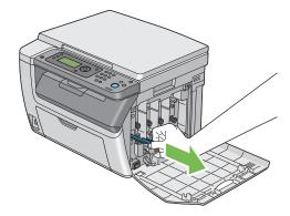
7 Insert the cleaning rod fully into the hole beside the arrow on the printer until its tip reaches the interior of the printer as illustrated below, and then pull it out.
