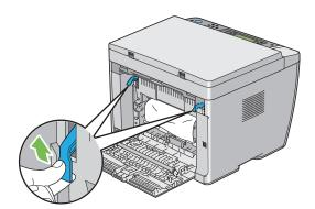
3 Remove any paper jammed from the back of the printer. If no paper is found in the paper path, face the front of the printer and check the center output tray.
