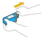
3 Adjust the toner cartridge to the associated cartridge holder, and then insert it firmly by pressing near the center of the label until the toner cartridge clicks.
