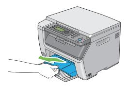
2 Remove any paper jammed from the front of the printer.
