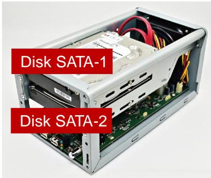
Repeat Step1~Step3 to install **Disk SATA-1** to the upper bay. Remember to connect **Disk SATA-1** with SATA data cable 1 shown in the illustration in Step 2
