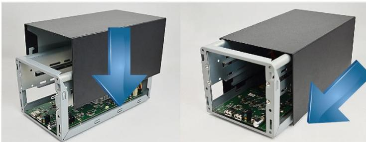
Install the case in reverse order of removal step (see Step 2), slide the case cover back until it clicks. Lock the back panel and then front panel with its screws.
