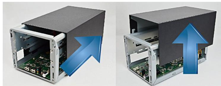
Slide the case backward until it stops, and then lift it up to remove.
