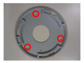
Tighten the plate to wall mount bracket with M4\*6 screws (not to use screws other than flat heads), and connect all necessary cables through the hole on the plate and wall mount kit
