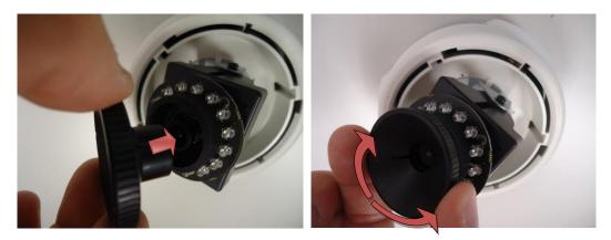
Remove the lens focus tuner.
