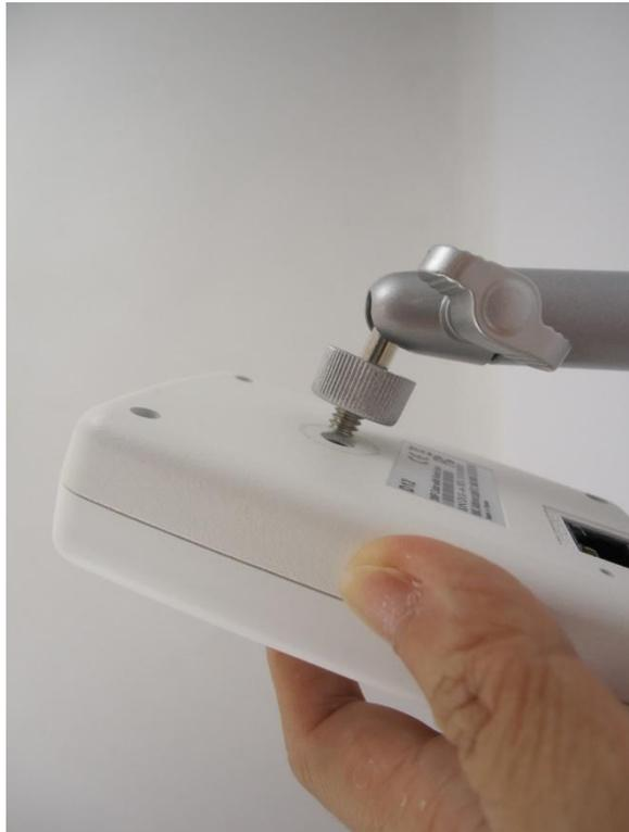
2. Position the camera to face the target view area.
