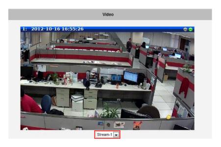
Usually, Stream-1 is configured to be high quality video with maximum resolution and frame rate for recording purposes while Stream-2 is usually a moderate quality stream for live view purposes of the VMS, to reduce VMS computing power during video decoding of multiple channels.
