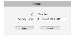
Similarly to UPnP, the human readable **Friendly Name** can be defined by the user. That name will be displayed when the camera is found in the network. By default, the Friendly Name is the serial number of the camera; however, the user can modify the name according to the project needs.
