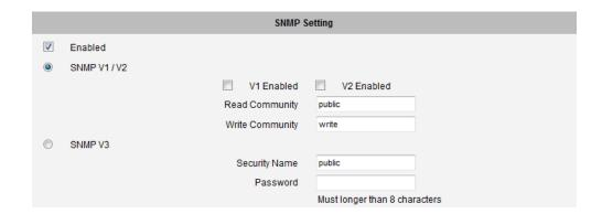
The SNMP agent supports versions V1, V2 and V3. SNMP V1 is the initial implementation of SNMP. SNMP V2 is proposed to enhance the performance of management, such as the communication of server and devices, the confirmation of information delivery and receipt. Primary additions in SNMP V3 concern security and remote configuration enhancements.
