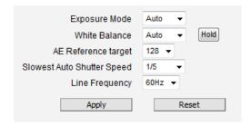
In Auto Exposure Mode, you control the image brightness by configuring the AE Reference Target and Slowest Auto Shutter.
